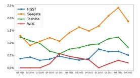
Figure 3: Failure Rate By Manufacturer
