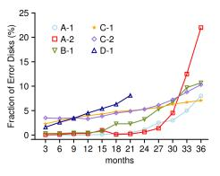
Figure 1: Percentage of disks developing sector errors. A-1 represents a specific disk model. As time progresses, although errors for each disk model are increasing, there are differences in the trend.
